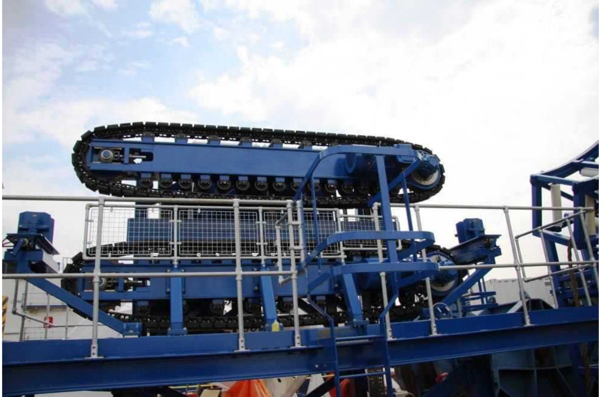
Example Aft Deck 10Te Side Loading 2 -Track Tensioner (on vessel)
