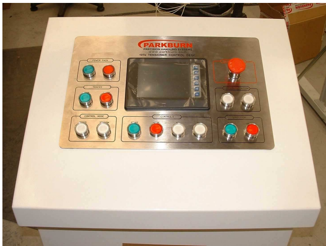
Example 10Te Tensioner Control Console
